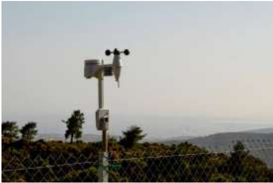
Figure 3: A weather station installed on the outskirts of the city provided data to the python program.
