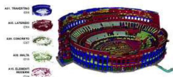
Figure 5: Example of material-based surface mapping.
