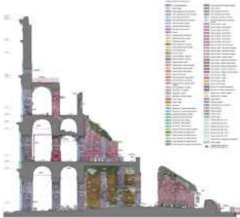
Figure 15: 2D restitution from the segmented point cloud, integrating undocumented information to provide a coherent reading of the building's constructive evolution.
