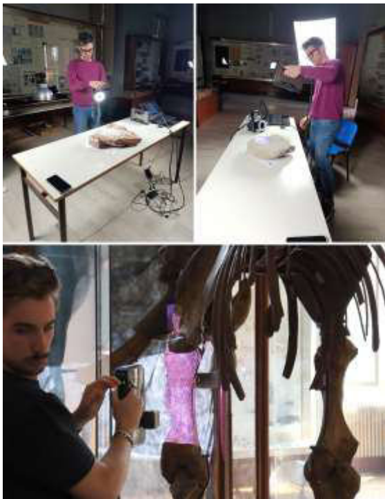
Figure 8: View of the objects digitization phases through photogrammetry and structured light laser scanner
