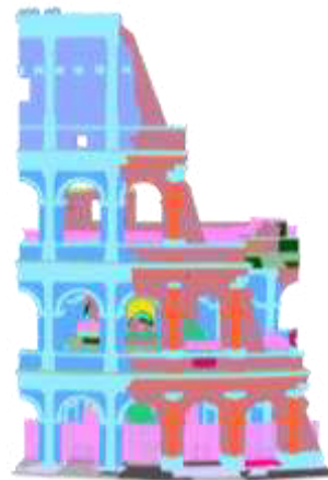
Figure 8: Portion of the point cloud with annotation of the pilot area’s materials
